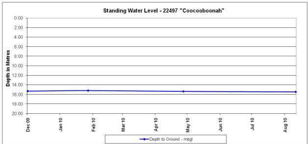
As discussed in the previous CCC report, results to date indicate minor variability in groundwater levels with no significant trend applicable. P5 is now located within the active pit area and monitoring bore 45098 has been covered by the waste dump and therefore both monitoring locations will no longer be sampled. Groundwater seepage into the pit is still minimal. Ongoing data collection will provide for longer term analysis of groundwater impact.
